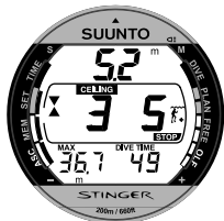
Fig. 3.13. Mandatory Safety Stop. You are advised to make a mandatory Safety Stop in the zone between the ceiling and floor.
