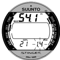
Fig. 4.9. Setting Oxygen Percentage and Partial Pressure.
