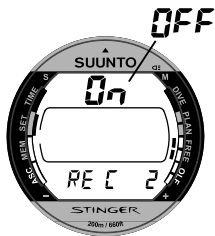
Fig. 4.11. The enable/disable status of the Free Mode and the recording rate setting.
