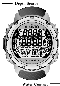
Fig. 2.2. The water contact and depth sensor.
