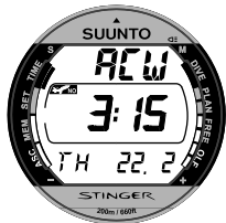
Fig. 2.3. Active water contact is indicated by the text ACW.
