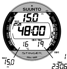
Fig. 3.35. Alternating display after Gauge dive. Center window showing the no-flying time.
