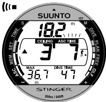
Fig. 3.17. Decompression dive, below floor. Upward pointing arrow, blinking ASC TIME label and an audible alarm tell you to ascend. Minimum total ascent time including safety stop is 7 minutes. Ceiling is at 3 m [10 ft].
