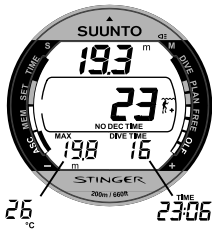
Fig. 3.11. Diving display. Present depth is 19.3 m [63 ft] and no-decompression stop time limit is 23 minutes in A0/P1 mode. Maximum depth during this dive has been 19.8 m [65 ft], elapsed dive time is 16 minutes. Alternative display shows temperature and current time.
