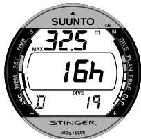
Fig. 5.9. Scuba Dive History Memory. Total number of dives, dive hours and maximum depth.
